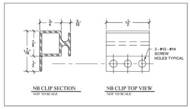
Model # VRSC NB: Primarily used in horizontal "No Batten" application. Use one fastener per clip for on stud application and two fasteners per clip for on sheathing application. The clip is 1.5" wide and allows for .75" air space behind siding.
